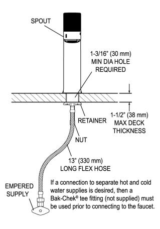
Thermostatic mixer ordered separately to comply with ASSE 1070 requirements. The product shall be tested and certified to industry standards: ASME A112.18.1M, CSA B125.1, California Health and Safety Code 116875
